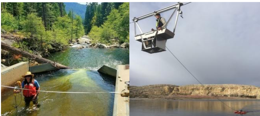
USGS scientists taking velocity and depth measurements
